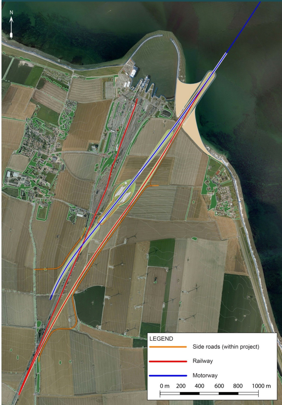
FIGURE 6.14 Conceptual design of a cable-stayed bridge – Outline proposal for alignment for road and railway, Fehmarn
