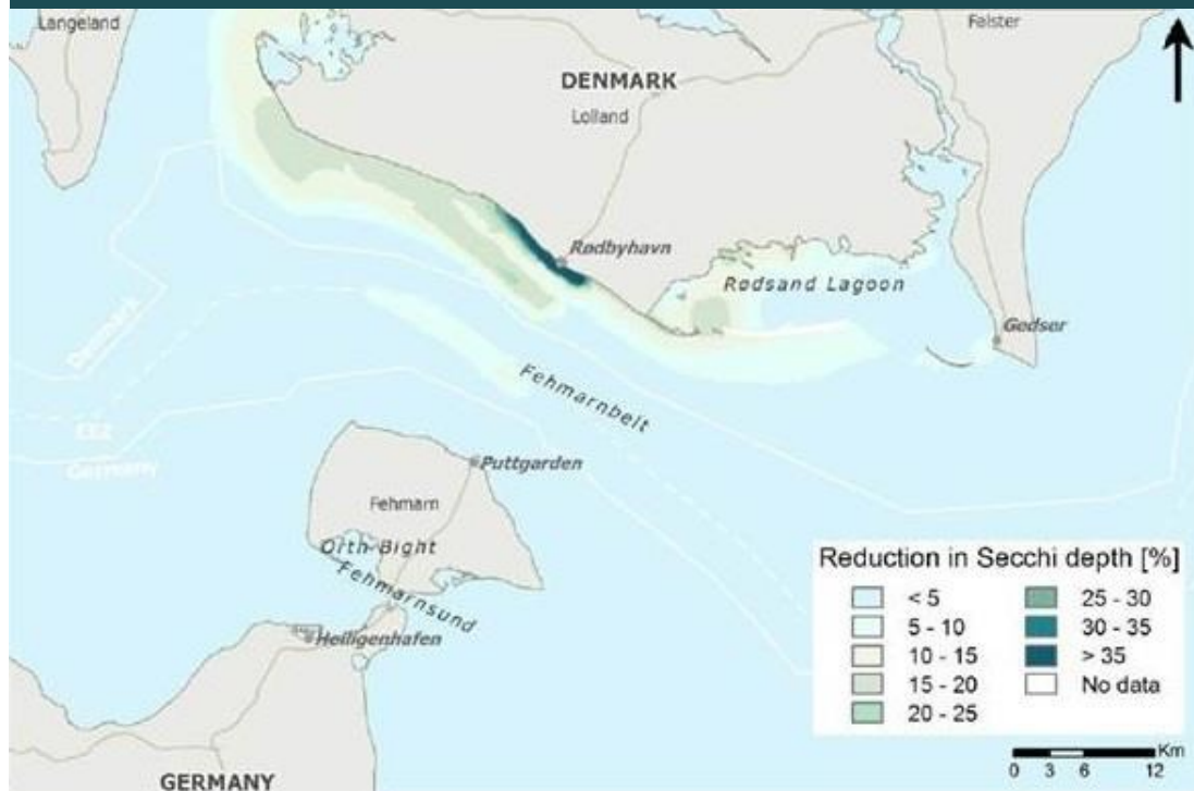
FIGURE 7.8.2 Modelled reduction in Secchi depth due to dredging within the first two years of construction period
