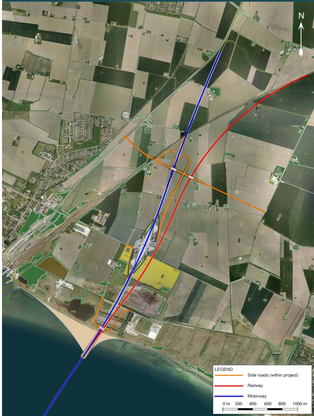
FIGURE 6.12 Conceptual design of a cable-stayed bridge – Outline proposal for alignment for road and railway, Lolland
