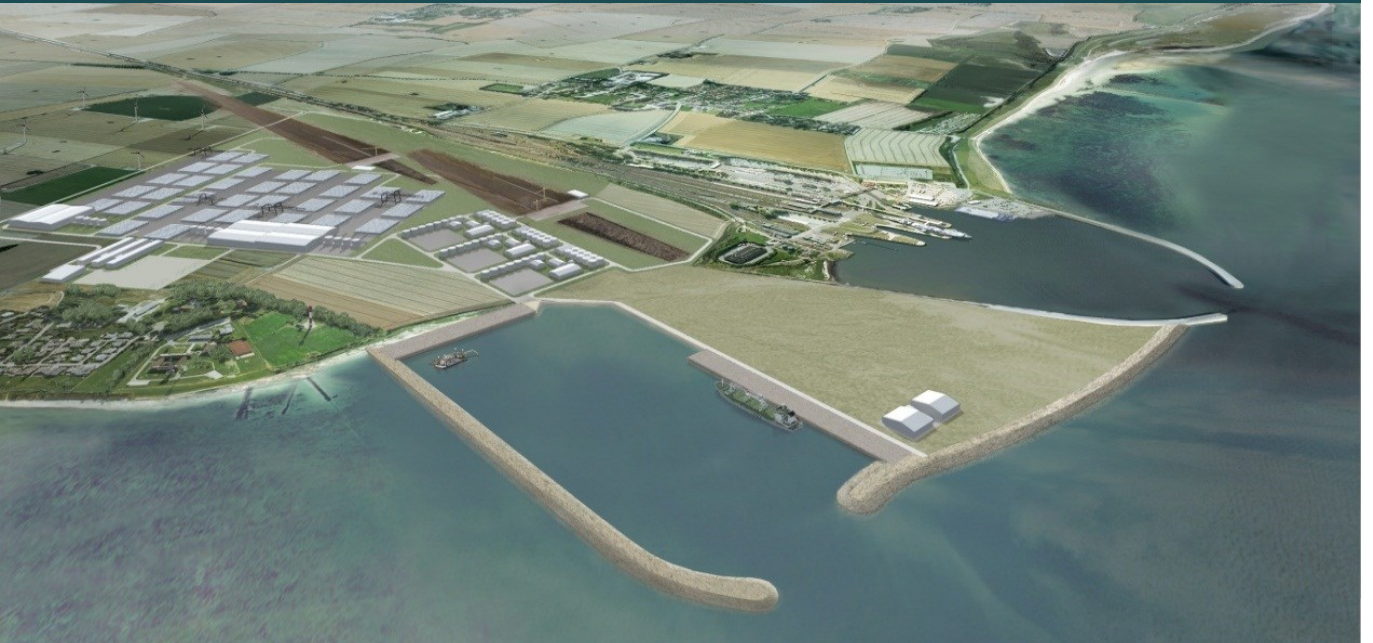
FIGURE 6.26 Conceptual design of bored tunnel – Illustration of the production area on Fehmarn
