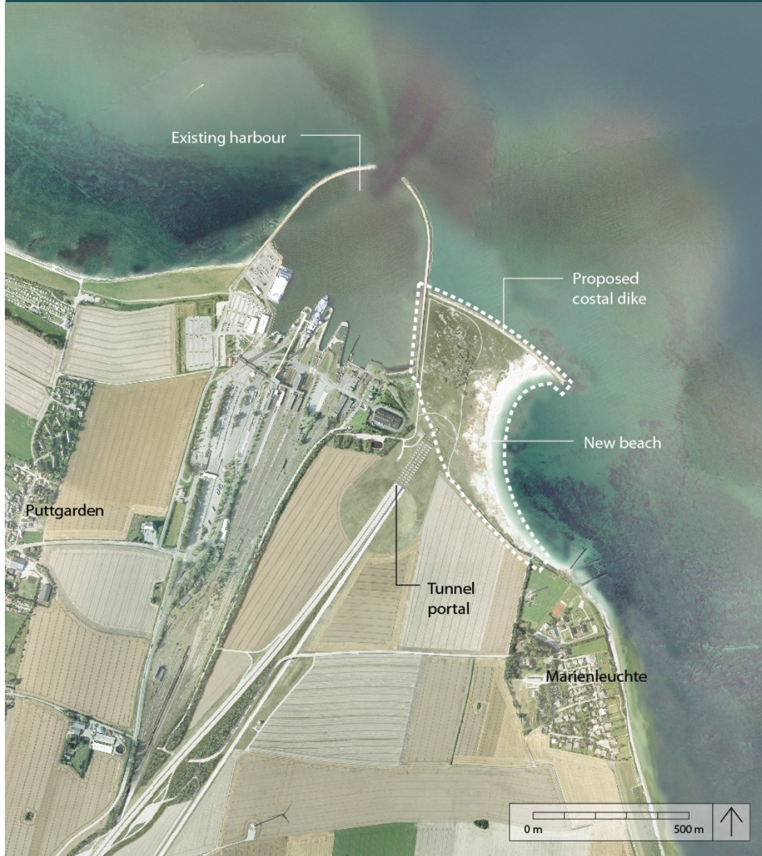
FIGURE 5.12 Conceptual design of an immersed tunnel – Design proposal for a land reclamation area on Fehmarn in Germany
