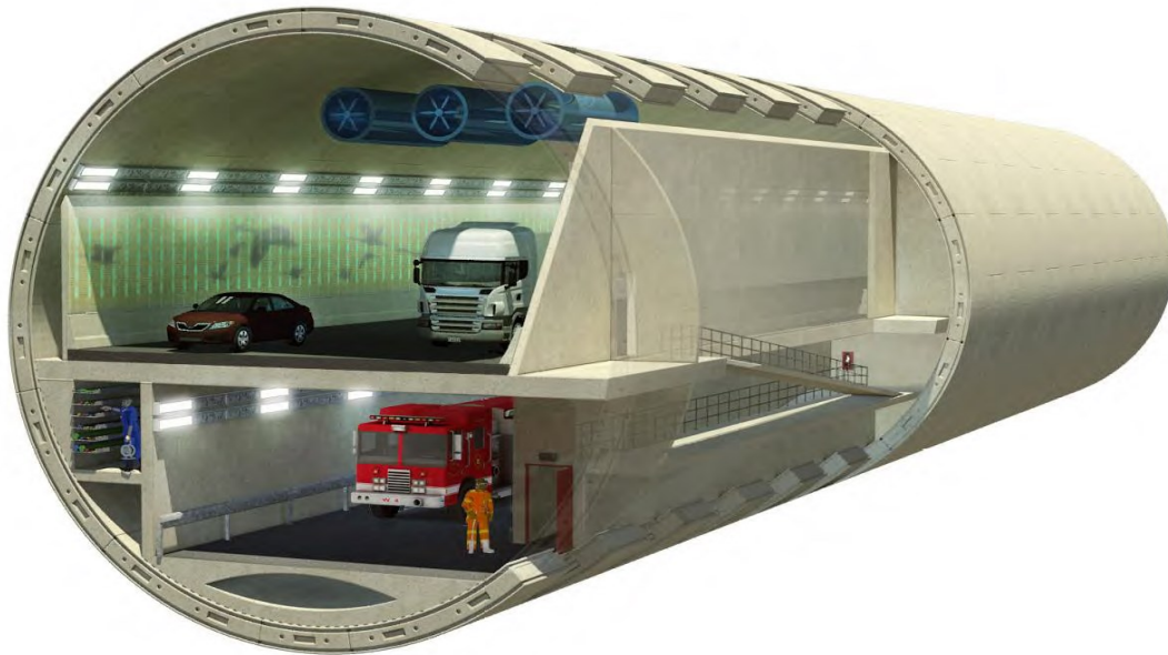
FIGURE 6.22 Conceptual design of a bored tunnel – Illustration of cross-section of the two motorway tubes
