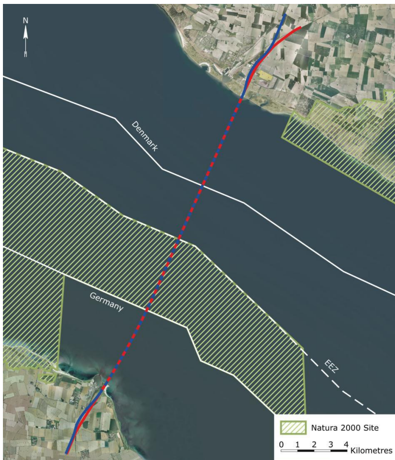
Figure 2.1 Proposed alignment for immersed tunnel E-ME (August 2011)
