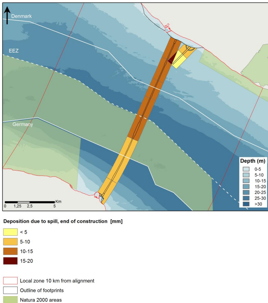
Figure 0.9 Sand deposition along the alignment of the tunnel
