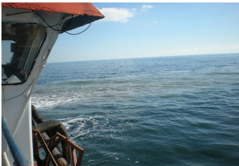
Figure 3.6 Sediment plume from field test October 2009. Concentration 3-4 mg/l. See Appendix P
