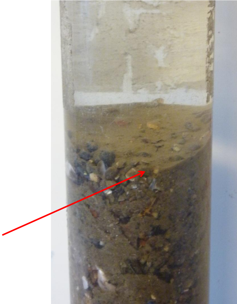
Figure 3.13 Seabed sample at NS03. The seabed consists of a very coarse material of sand and gravels but on the day overlaid with about 1mm thin layer of very fine material (red arrow)
