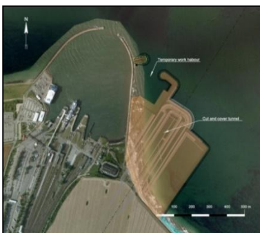
Figure 6.2-4 Fehmarn temporary harbour
