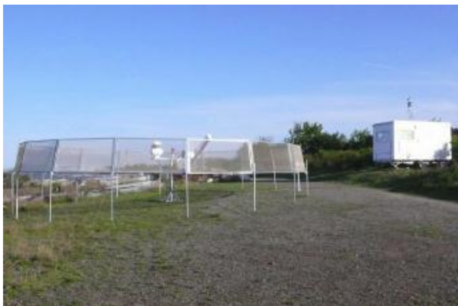
Figure 3.2 Field station Puttgarden with dual radar, clutter fence and trailer.
