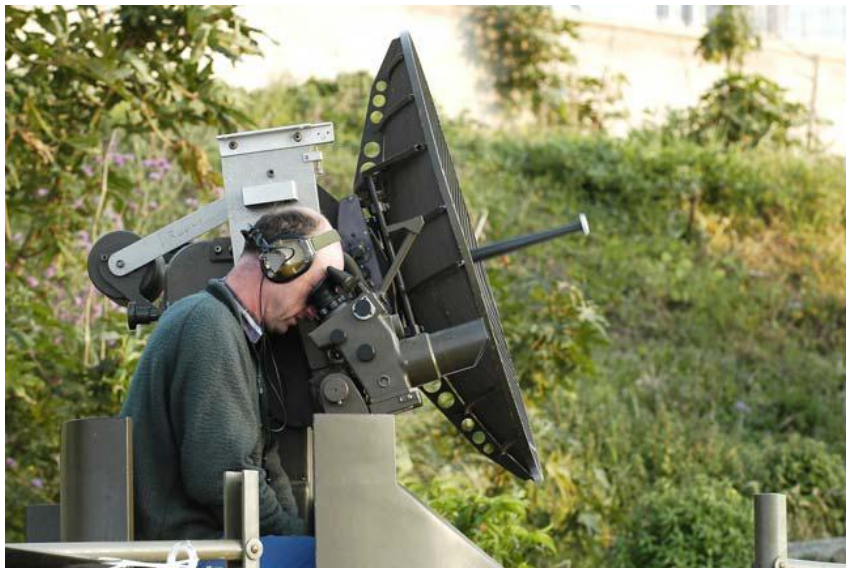
Figure 3.13 The observer on the radar tower identifies birds flying in the radar beam with the telescope mounted parallel to the axis of the beam.
