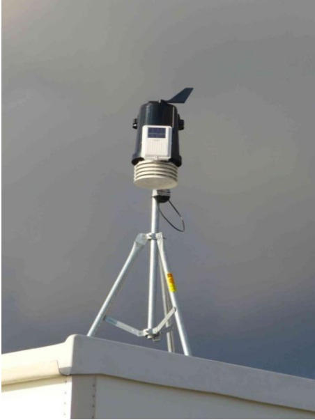
Figure 3.14 Weather station used on land stations, mounted on the roof of field station trailer.
