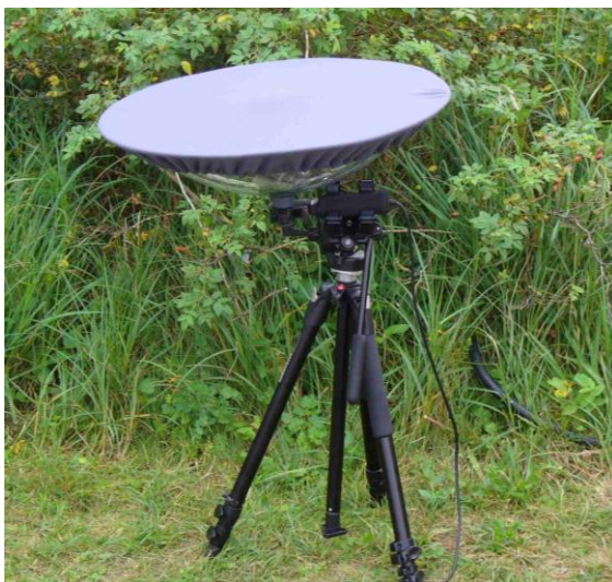
Figure 3.8 Parabolic dish with microphone inside.
