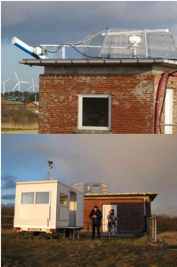
Figure 3.3 Field station Rødbyhavn with dual radar and clutter fence mounted on the roof, trailer and weather station.
