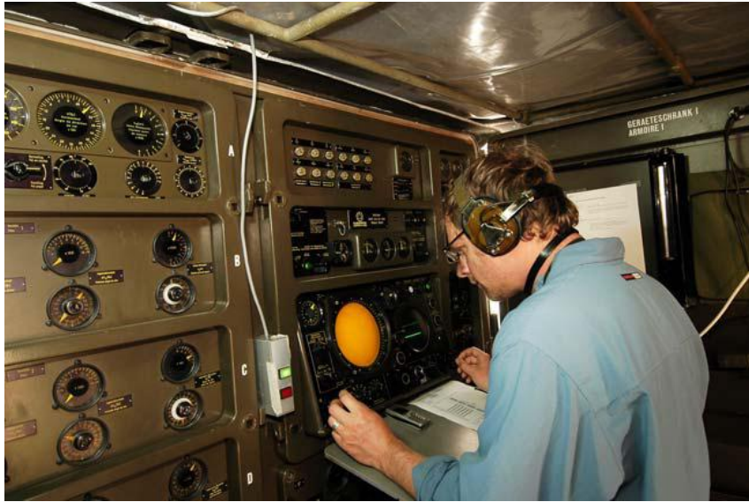
Figure 3.12 The radar operator searches birds on the screen and assigns them to the radar for tracking.
