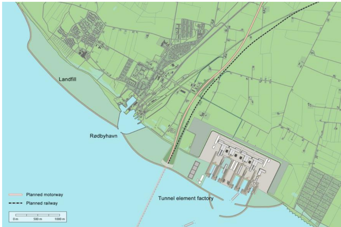
Figure 2.7: Proposed lay-out of the production site on Lolland. © Femern A/S
