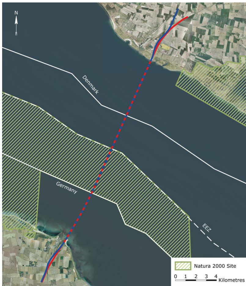
Figure 2.1: Proposed alignment for immersed tunnel E-ME (August 2011). © Femern A/S
