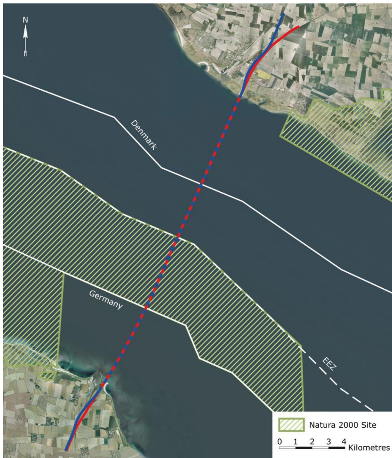
Figure 2.1 Proposed alignment for immersed tunnel E-ME (August 2011).
