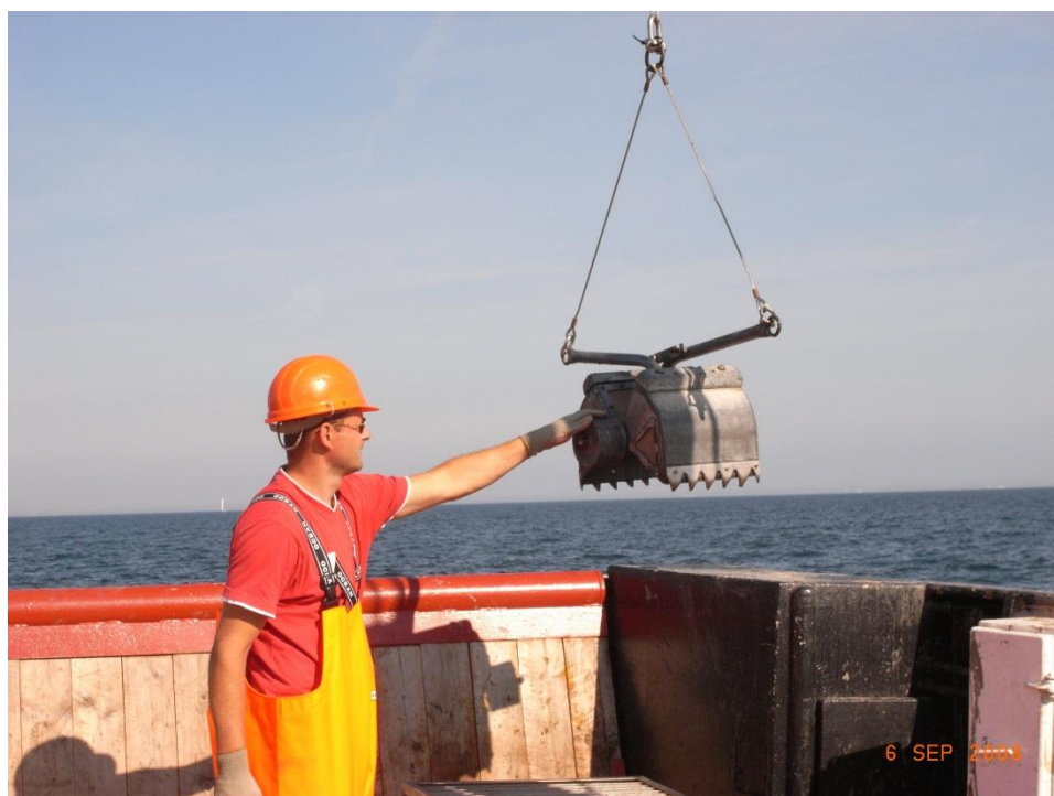
Figure 2-5 A Van Veen grab sampler, operated with a large winch, from a ship. The grab sampler is used to sample sediment and benthic infauna in the deep waters below the pycnocline.
