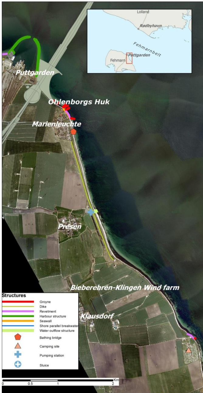
Figure 5.13 New permanent structures along the Fehmarn coast in the tunnel project – east of Puttgarden. Aerial photo from 2009 (©COWI Orthophoto April 2009). Note: Biéberehren-Klingen wind farm is not the correct name of the wind farm south of Presen
