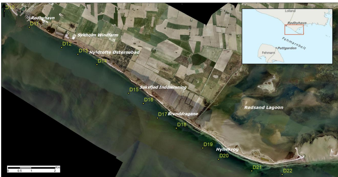
Figure 3.12 D1-D22: locations of coastal cross sections for analysis of nearshore wave climate. D6-D17: coastal cross sections where littoral drift has been calculated. Lolland coast. Aerial photo from 2009 (©COWI Orthophoto April 2009)
