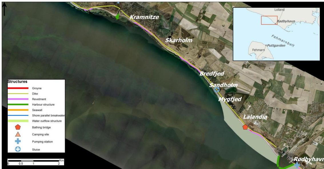
Figure 5.1 New permanent structures along the Lolland coast in the tunnel project – west of Rødbyhavn. For enlarged version of this figure, refer to Figure 6.1. Aerial photo from 2009 (©COWI Orthophoto April 2009)
