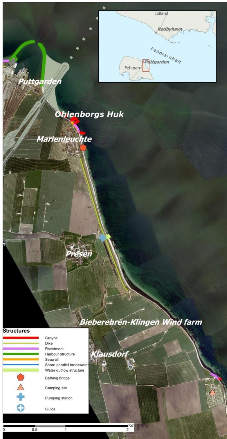
Figure 7.4 New permanent structures along the Fehmarn coast in the bridge project – east of Puttgarden. Aerial photo from 2009 (©COWI Orthophoto April 2009) . Note: Bieberehren-Klingen wind farm is not the correct name of the wind farm south of Presen
