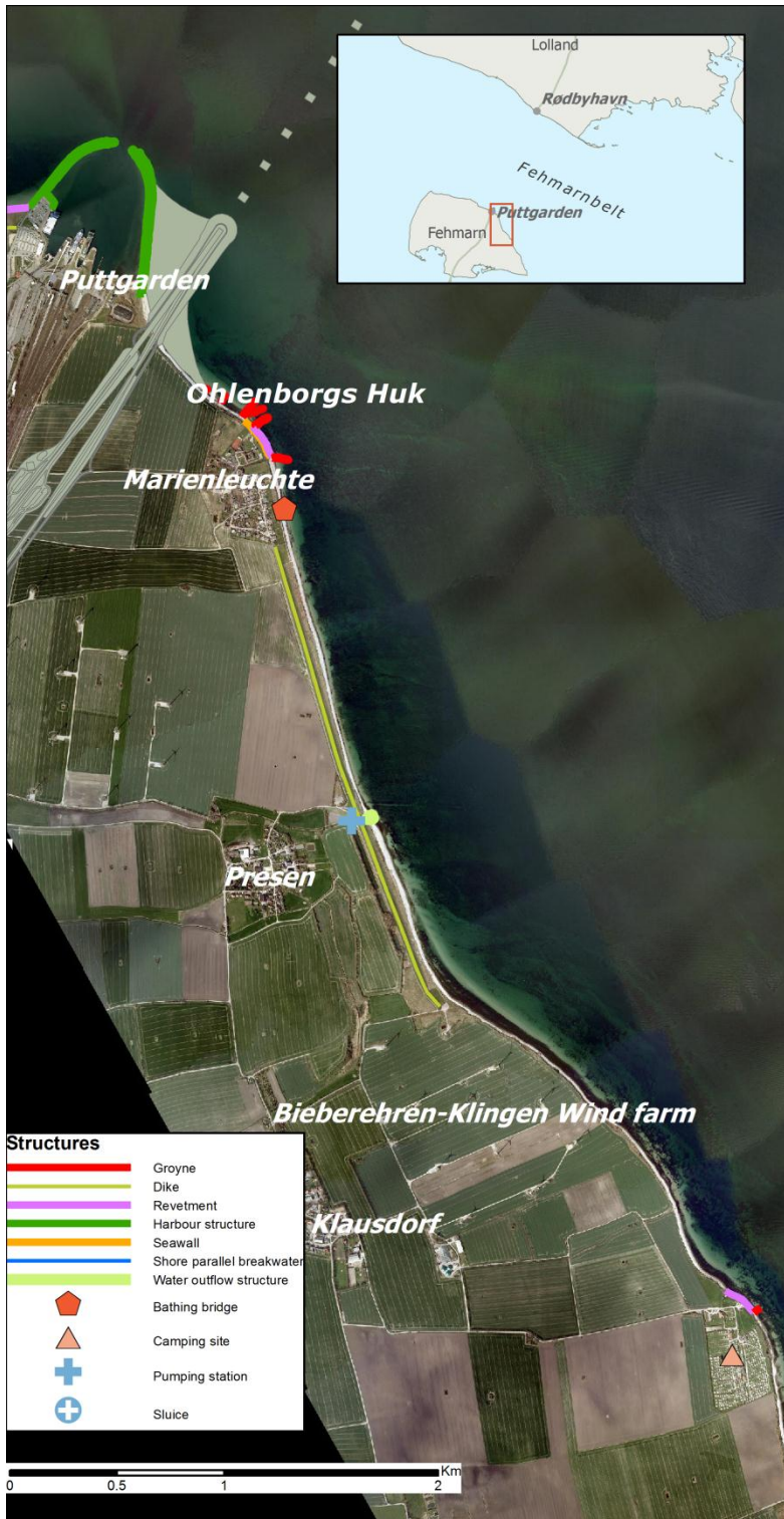
Figure 5.31 New permanent structures along the Fehmarn coast in the bridge project – east of Puttgarden. Aerial photo from 2009 (©COWI Orthophoto April 2009). Note: Bieberehren-Klingen wind farm is not the correct name of the wind farm south of Presen
