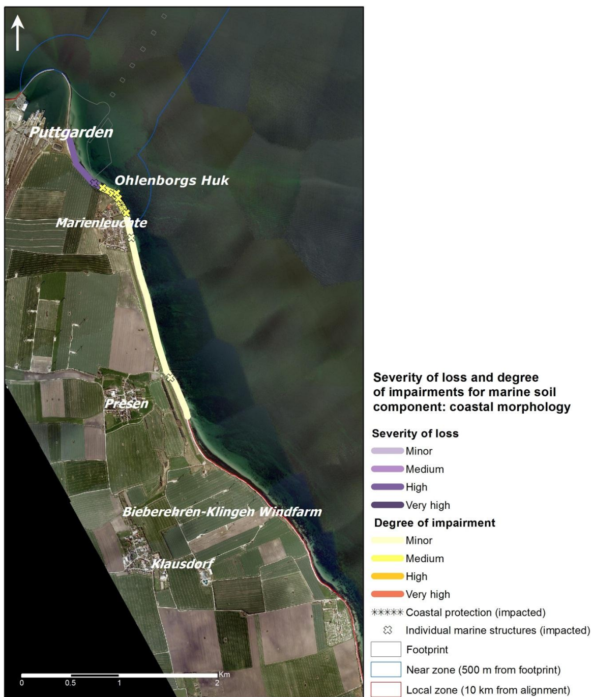
Figure 7.7 Degree of impairment and severity of loss assigned to sections of the coast of Fehmarn southeast of Puttgarden due to the pressure from the bridge project. Note that legends for structures along the coast (coastal protection and individual marine structures) are shown on top of signs for loss/impairment. These indicate hence the loss of and degree of impairment for such structures. Note: following this assessment, additional planned mitigation measures have been included. The impairments to coastline and structures southeast of Puttgarden will hence not become effectuated, please refer to the text. Aerial photo from 2009 (©COWI Orthophoto April 2009). Note: Bieberehren-Klingen wind farm is not the correct name of the wind farm south of Presen
