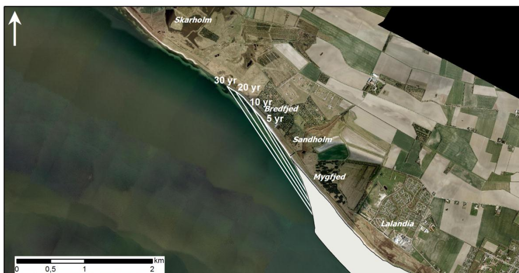
Figure 6.4 Predicted development of shoreline west of the Lolland reclamation 0-30 years after end of construction. Aerial photo from 2009 (©COWI Orthophoto April 2009)
